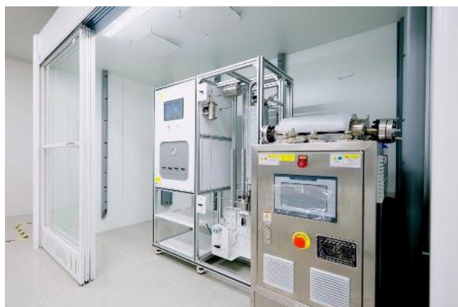
Figure 2. Continuous hydrogenation with fixed bed reactor in pilot production scale
