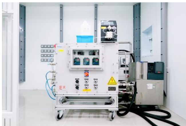
Figure 4. Photochemistry reaction with the Plug Flow Reactor (PFR) systems
