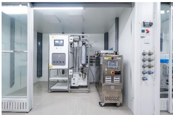
Figure 2. Continuous hydrogenation with fixed bed reactor in pilot production scale
