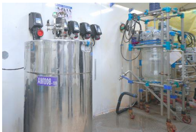
Figure 1. Ozonolysis reaction with the low temperature conditions in Continuous Stirred Tank Reactor (CSTR) systems
