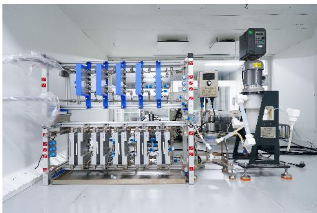
Figure 3. Two phase fast reaction (less 10s) with Microchannel systems
