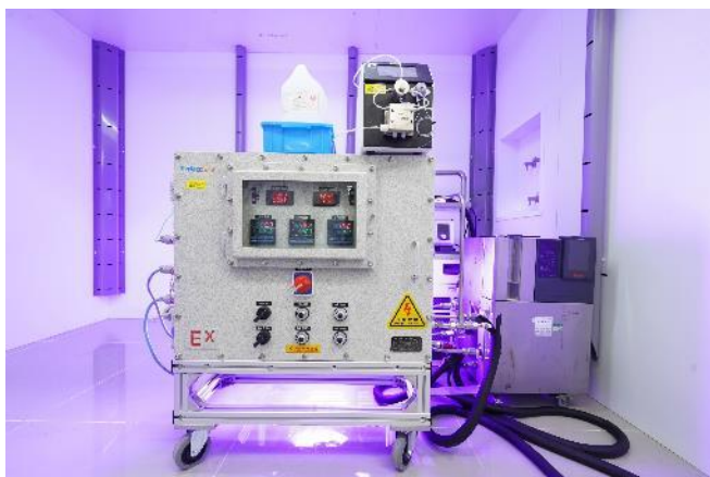
Figure 4. Photochemistry reaction with the Plug Flow Reactor (PFR) systems
