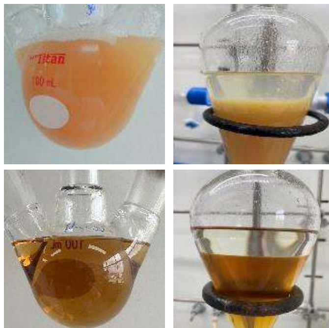
Figure 4. Comparison of reaction slurry and extraction: free enzyme process (upper), immobilized enzyme process (lower).
